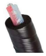
A Contact python line is a group of multiple tubes bundle covered with insulation foam to dispense beverages like beer, softdrinks, spirits, etc. at low temperatures. A good python is designed to slow down the heat input thus preventing from drinks to warm up when the taps are not being used. The insulation foam reduces the heat gain and the water recirculation lines take heat of the python thus maintaining a low bundle temperature.
